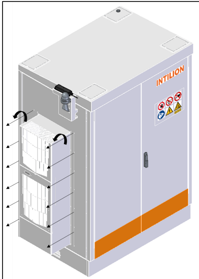
Fig. 55 Battery storage – remove screws
